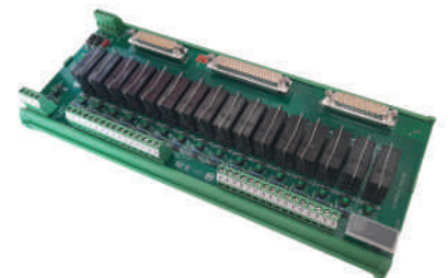
16 Channel DI Relay module with DI redundancy and one pot free contact on D sub connector
